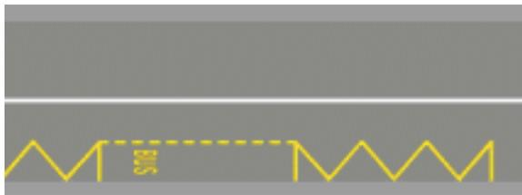
The signs in the figure indicate an area for the stop of buses, trolleybuses and articulated buses in public service, and are used by buses to facilitate the approaching maneuver and to restart.
