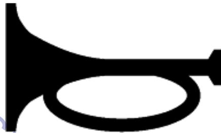
**Ye acoustic signaling device ki command ko zahir krta hai. Ye kisi warning light se connected nai hai.**
